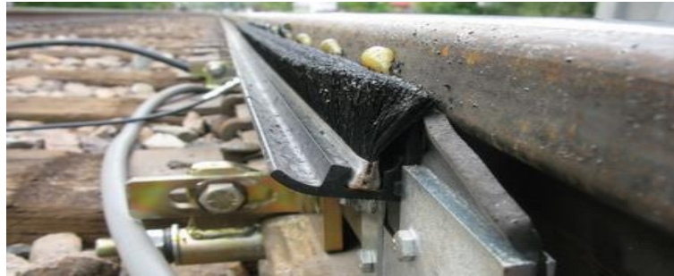
Figure 4. An example of the wayside lubrication systems for gauge face [10]
