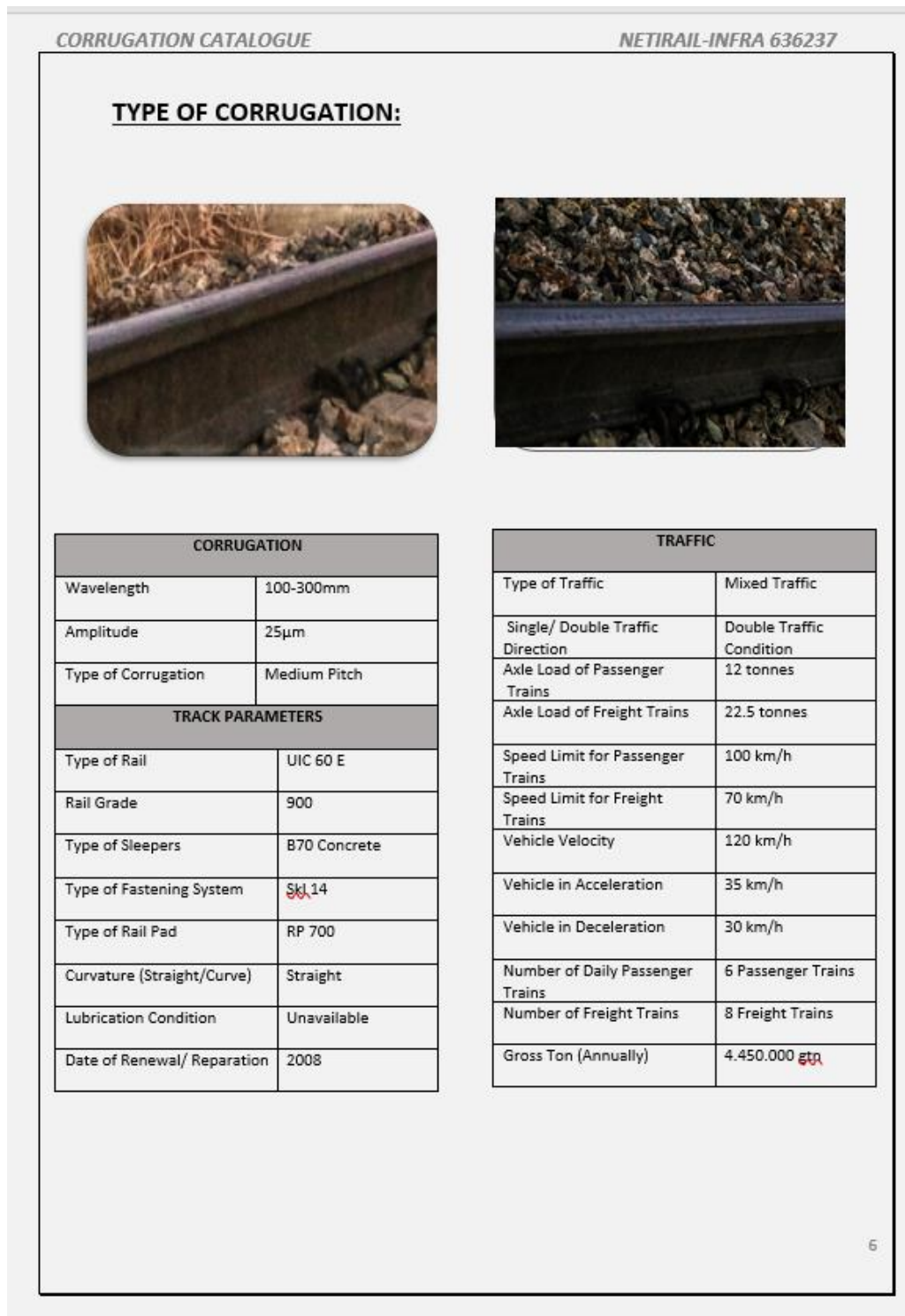
Figure 2.2.2 An example of TCDD corrugation catalogue (medium pitch corrugation)
