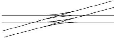
Figure 1.15 - A diamond crossing with inside double slip
