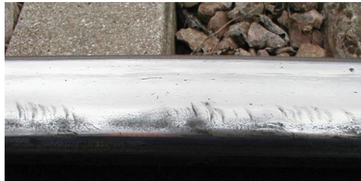
Figure 1.20 - Head checks at the surface of a rail gauge corner (Cannon et al., 2003).
