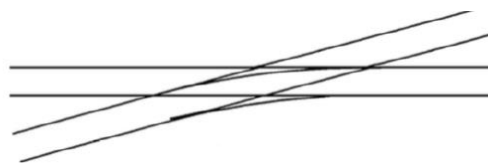
Figure 1.13 - A diamond crossing with inside single slip
