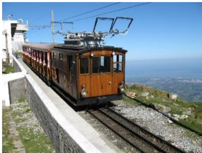
Figure 2.5 – Train using a multiphase electrification system, with multiple pantographs, on the Petit trains de la Rhune, France
