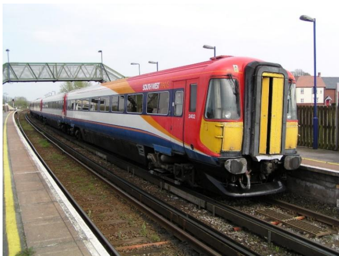
Figure 3.17 – British Class 442 third rail electric multiple unit in Dorset; this is the fastest class of third rail EMU in the world, reaching 172 km/h
