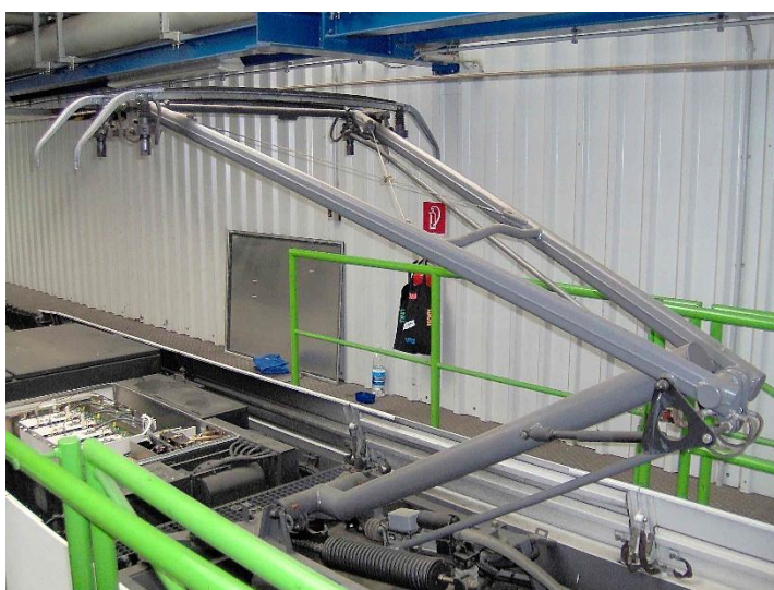
Figure 3.6 – The (asymmetrical) 'Z'-shaped pantograph using a single-arm design
