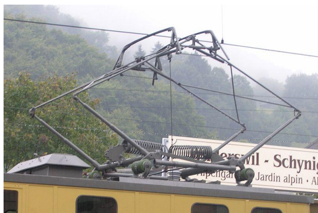
Figure 3.7 – Symmetrical, diamond shaped pantographs of the Swiss cogwheel locomotive of the Schynige Platte railway
