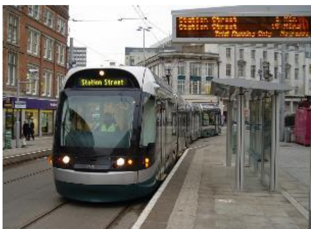
Figure 2.3 – Nottingham Express Transit in United Kingdom uses a 750 Vdc overhead, in common with tram systems 1
