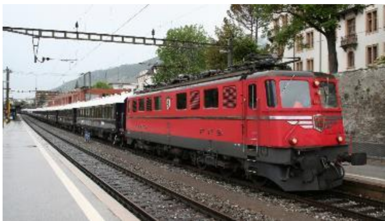
Figure 2.4 – 15 kV 16.7 Hz AC traction current used in Switzerland 2
