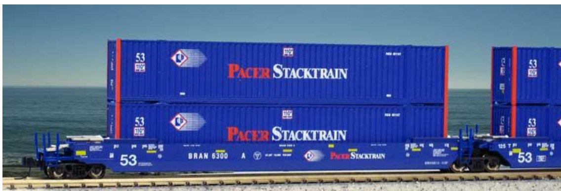
Figure 3.1 – Most overhead electrification do not allow sufficient clearance for a double-stack car 4
