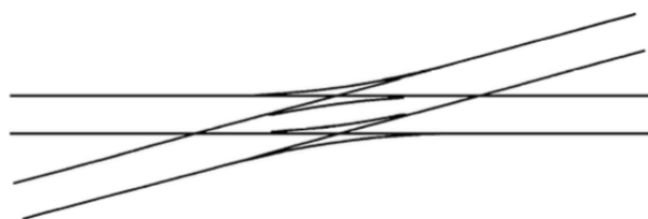
Figure 2.12 - A diamond crossing with inside double slip
