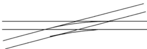
Figure 2.10 - A diamond crossing with inside single slip
