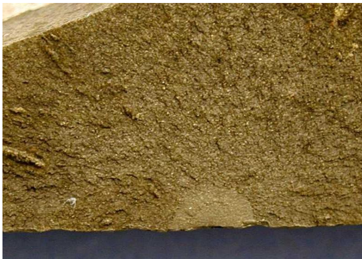
Figure 1.19 - Rail breakage from a fatigue crack initiating at a corrosion pit 15
