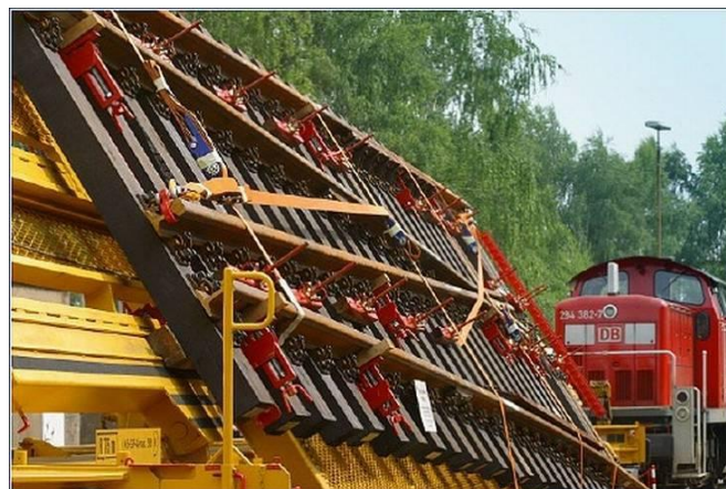
Figure 2.11 - Tilting wagons used to transport switch panels from factory. (Source: DB).
