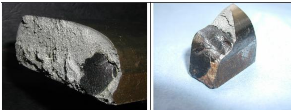
Figure 1.18 - Example of a Sub-surface Initiated RCF Crack 14
