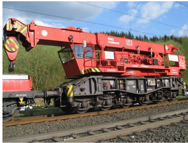
Figure 2.10 - Multi-purpose railway crane commonly employed for switch renewal. (Source: DB).
