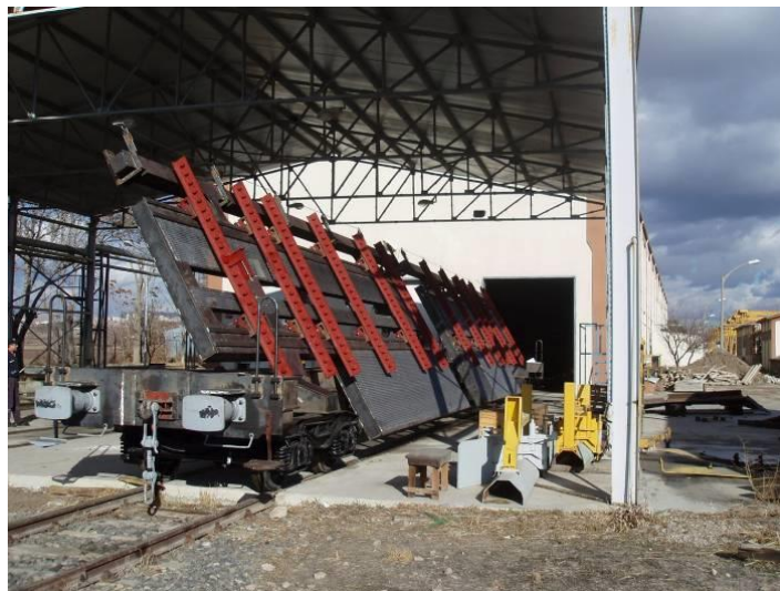
Figure 2.18 - TCDD tilting wagon for switch panel transport (source: TCDD).
