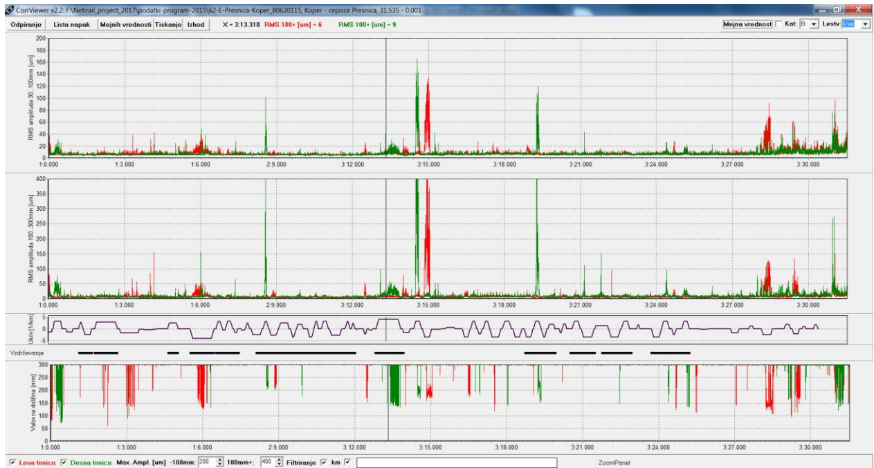
Figure 6.7: Corrugation diagram for line 62E cepišče Prešnica-Koper in 2015.
