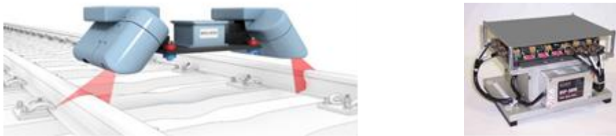
Figure 5.5: Line geometry measuring system on the track inspection machine.
