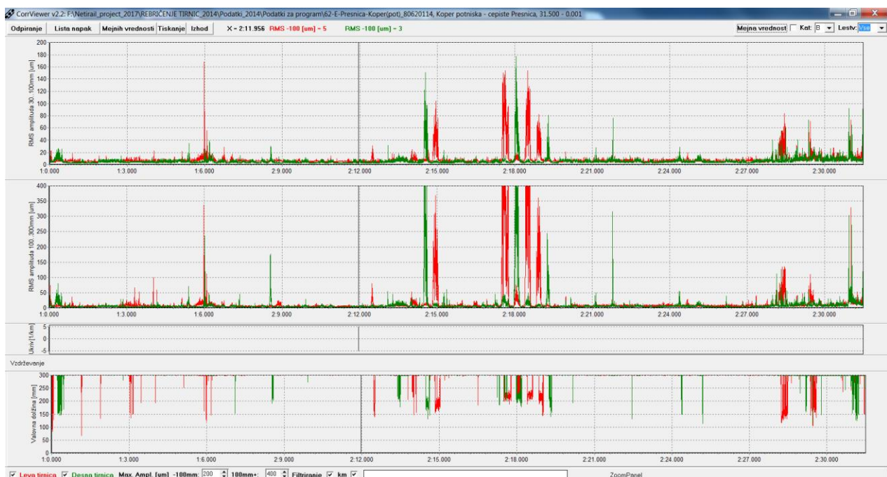
Figure 6.6: Corrugation diagram for line 62E cepišče Prešnica-Koper in 2014.
