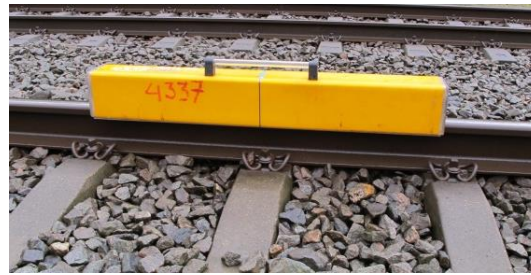
Figure 2-4. RAILPROF measurement of rail corrugation longitudinal profile
