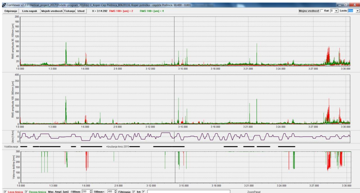
Figure 6.8: Corrugation diagram for line 62E cepišče Prešnica-Koper in 2016.
