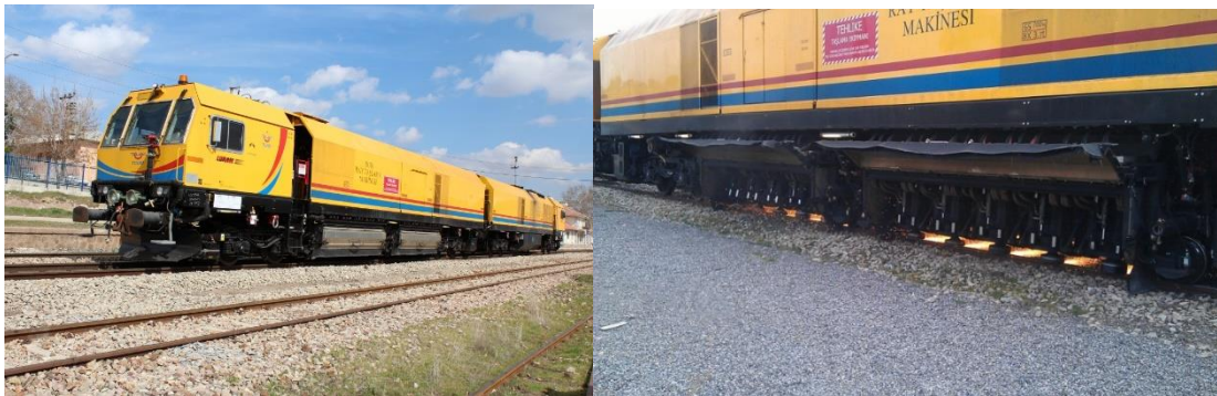
Figure 5.7: Rail grinding machine.
