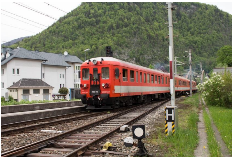
Figure 6.3: Measuring train MAV AB25-SDS-AB35
