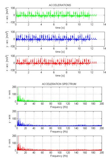
• Even the actuator provides displacement on the OZ axis, the energy and displacements are spread on all three axes
